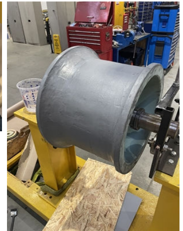
Build up of Belzona 1111
