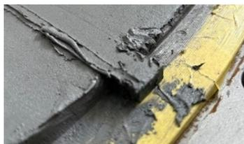
Belzona 1511 rebuild reforming separator channel.
