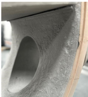
Pitting damage of Water Box after grit blasting.
