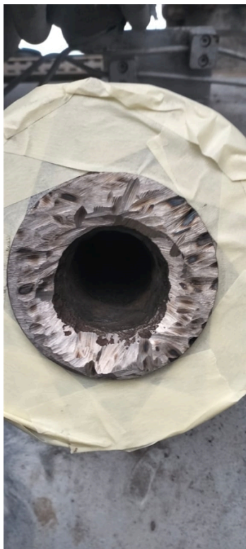
Surface preparation is done over the flange face before the rebuilding
