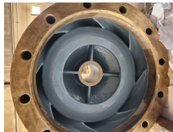
Second coat of Belzona 1391T on the pump discharge head
