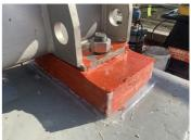
Screw press requires a high-performance chocking at the support legs to ensure stability and minimize vibrations
