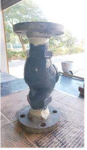
Globe valve that had developed After thorough cleaning, the a hole, leading to operational disruptions.
