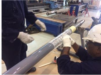
The first coat of Belzona 1321 (Ceramic S-Metal) was applied.
