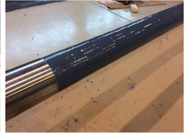
Finally, two coats of Belzona 1321 (Ceramic S-Metal) were applied, following the Belzona Instructions for Use (IFU), to provide superior protection and long-term performance.
