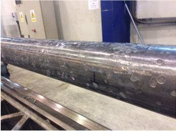
Severe pitting on the exposed section of a vessel's tail shaft due to prolonged seawater exposure and barnacle adhesion
