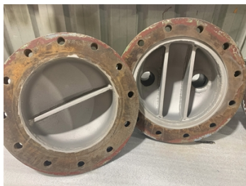
End covers were blasted for further repair steps
