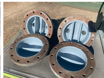
End covers completed with second coat Belzona 1391T Blue
