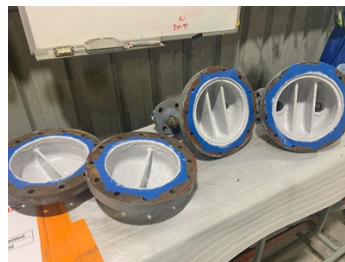
First coat of Belzona 1391T Grey
