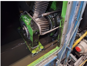
Gearbox with damaged bearing
