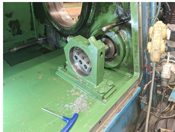
Treatment of damaged surface prior to application of Belzona 1111
