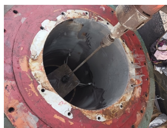
Machining down to required dimensions.
