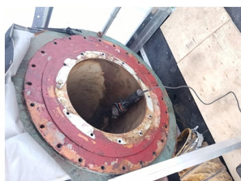
Stern tube after cleaning.
