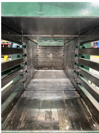
Baler lining after power tool cleaning before application of Belzona 1121.
