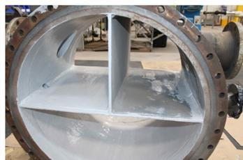
After the components are reprofiled using Belzona 1511, the first coat of Belzona 1391T is applied
