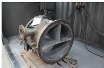
Components are grit blasted back to expose eroded areas and produce a minimum surface profile
