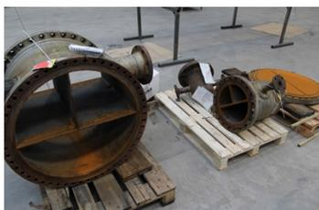
Heavily eroded heat exchanger components were in need of repair
