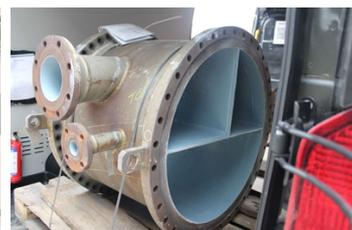
Two coats of Belzona 1391T and the components are protected against erosion and ready to go back into commission
