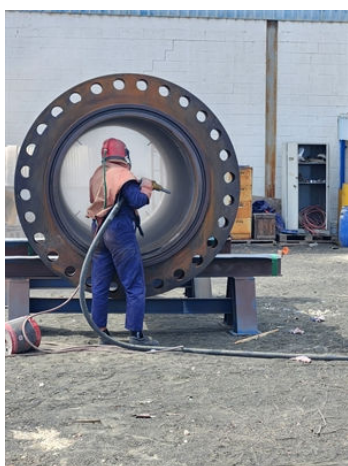
Surface preparation to reach a minimum profile of 75 µm and near white metal
