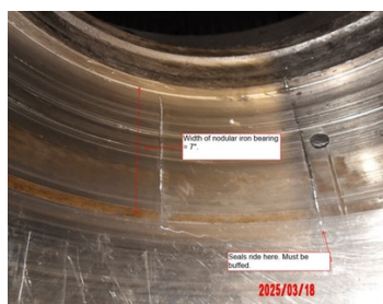
View and dimensions of some of the damaged sections
