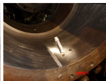
Thinner gouges filled and sanded
