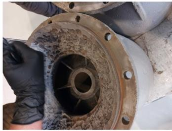
Rebuilding started using Belzona 1111 application by short bristle brush
