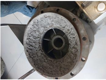
Bowl 1 Corrosion blasted and ready for rebuilding with Belzona 1111
