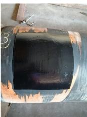
Floating hose was damaged due to collisions with ships and and power tool boats
