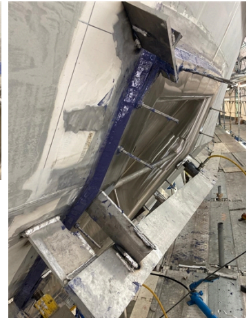
Finished application of Belzona 7311.
