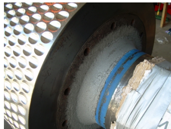
Surface prepped and ready for Belzona product
