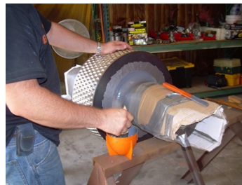
Applying Belzona 1391HT
