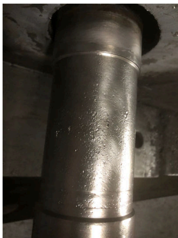
Close up of the pitting corrosion
