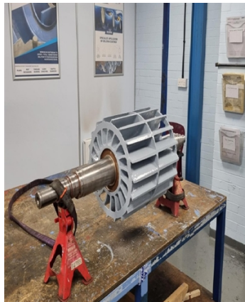
After Belzona 1111 has been applied to rebuild and first coat of Belzona 1341
