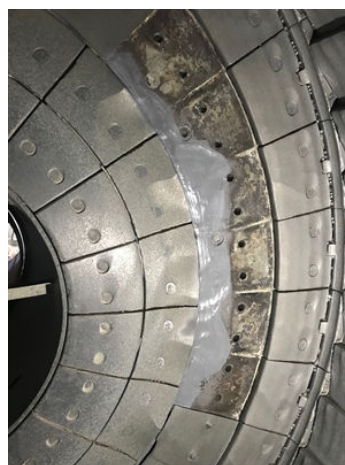
Same area as Photo 1, but now filled and ready for installation of wear plates
