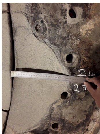
Showing depth of wear against Applications Team Straight edge
