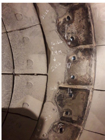
Showing large area of wear, once the wear plates have been removed
