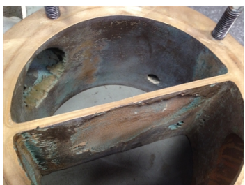
Degraded heat exchanger due to corrosion.
