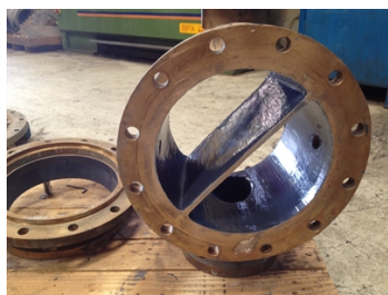
The equipment was subsequently coated with two layers of Belzona 1391(Ceramic HT) to ensure long-term protection.
