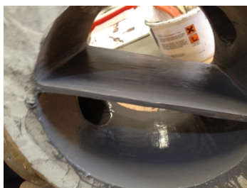
After cleaning the surface with Belzona 9111 (Cleaner Degreaser), Belzona 1311 (Ceramic R-Metal) was used to rebuild the damaged areas.
