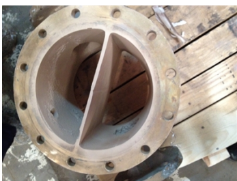
Surface preparation was done through grit blasting to SA 2.5 standard.
