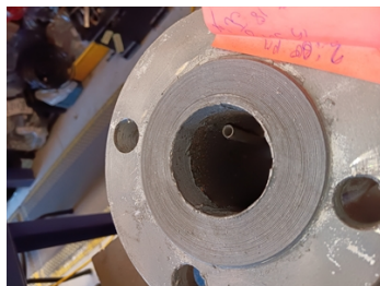
Flange face rebuilt using Belzona 1511, 9411 with customer supplied former.
