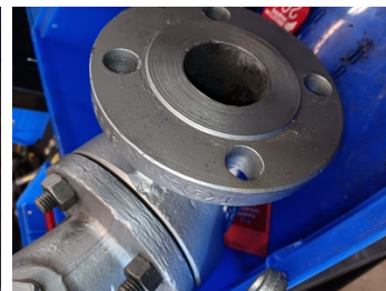
Rebuilt raised flange face complete and ready for installation and back into service.
