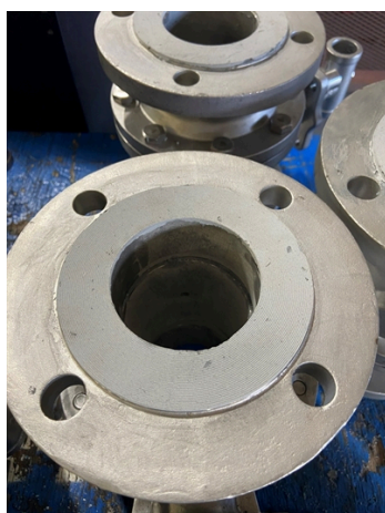
Close up picture on the flange after Belzona 1111 is applied and cured.
