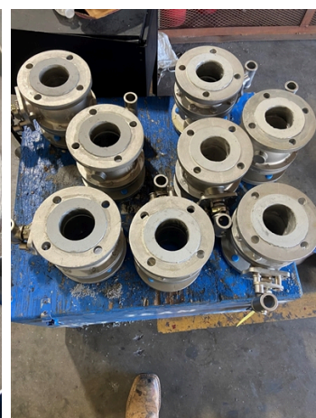
A number of flanges all rebuilt with Belzona 1111.
