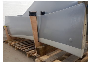
4. Closer detail of finished LEP and full body protection coating
