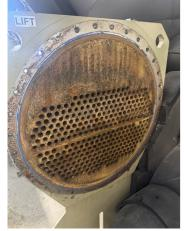
Initial condition of the heat exchanger showing severe corrosion and rust accumulation on the tube sheet surface.
