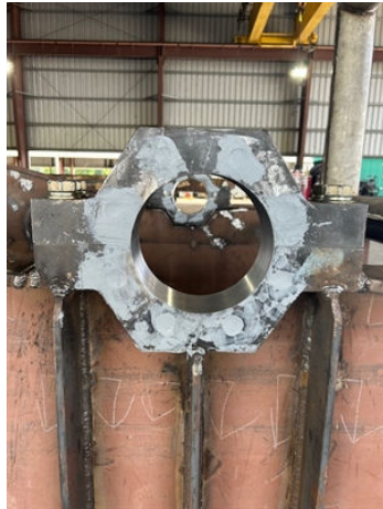
Holes filled with Belzona 1161 by injection.
