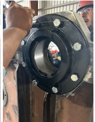
Bearing casing fit-tested for installation.
