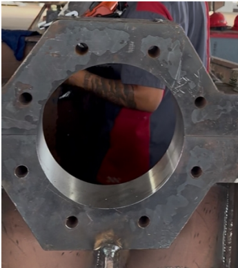
Pillow block with oversized bolt holes.
