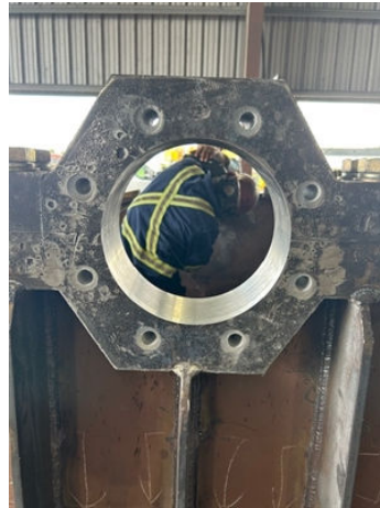
Holes bored to correct size through the Belzona 1161.
