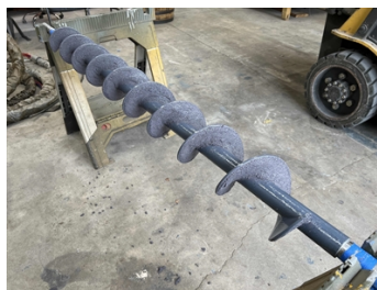
Applied Belzona 1812 (Ceramic Carbide FP) to the leading edges.
