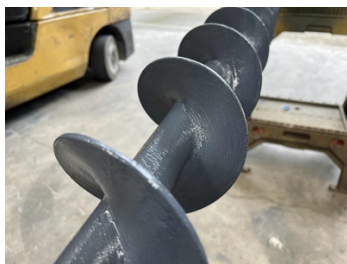
Belzona 1321 (Ceramic S-Metal) applied by stiff-bristle brush.
