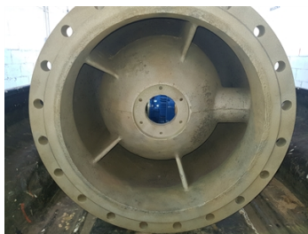
Valve body assembly arriving for preparation and application
