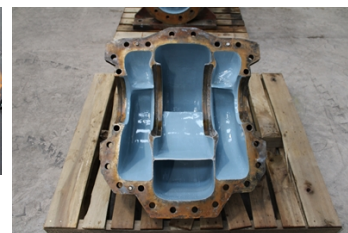
Two coats on Belzona 1391T are applied to protect against erosion/corrosion at high temperatures under immersion
