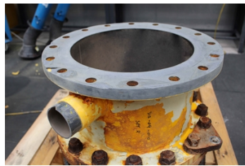
Water cooling spools arrive with damage to sealing faces and stabbings
