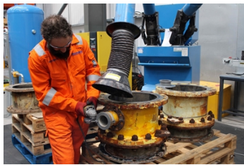
The surface areas are prepped to a minimum surface profile for the repair solution
