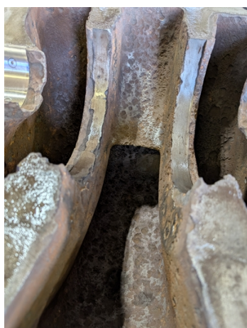
Severe pitting in the pump housing
