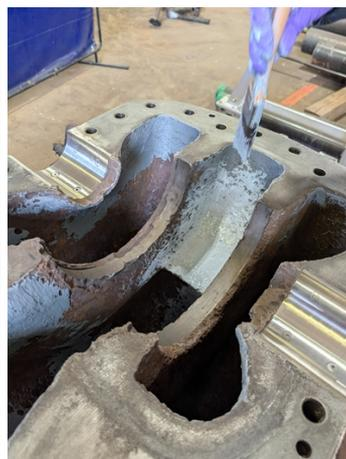
Rebuilding with Belzona 1121
