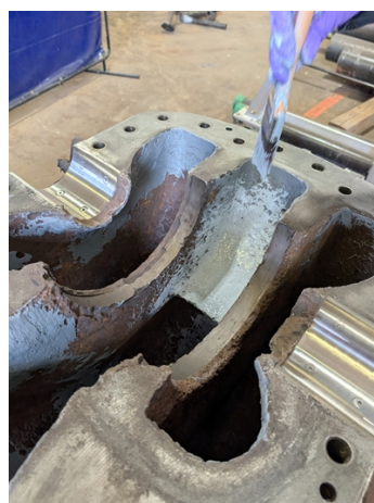
Rebuilding with Belzona 1121
