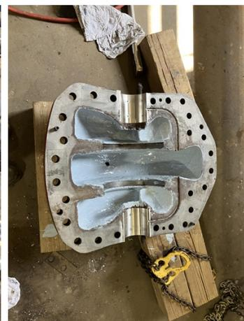
The pump house after the application of Belzona 1341
