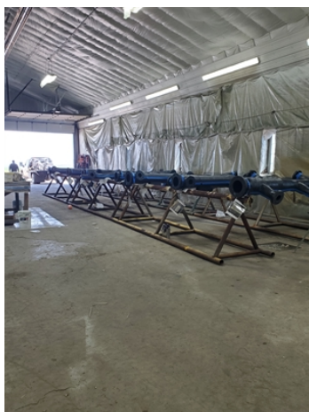
Fiberglass headers ready for manual preparation. These headers were taken off site and delivered to contractor's shop.
