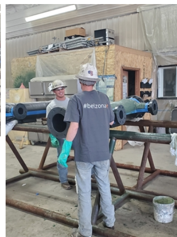
Belzona 1813 applied to fiberglass headers.
