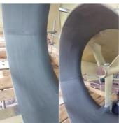
Surface preparation prior to the Surface rebuilding by Belzona 1311 (Ceramic R-Metal)
