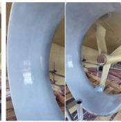
Kort nozzles are further protected by Belzona 1341 (Supermetalglide) coating.
