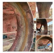
Kort nozzles condition suffers severe metal loss and require Belzona application
